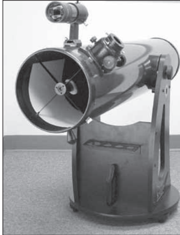
Figure 23. The SkyQuest optical tube properly set up for collimation. Note the white paper placed across from the focuser, and the level angle of the optical tube. Ideally, the telescope should be pointing at a white wall. (IntelliScope model shown.)
