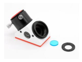
When the retaining ring is removed, the old blue-glass can be removed. If necessary, you can now remove silicone residues or dust. Now insert the new blue-glass and screw the retaining ring back in.
