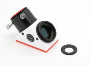
Now the retaining ring can be unscrewed counterclockwise, for example with a compass/circle or similar tool.
