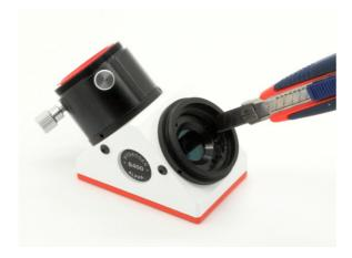
There is a retaining ring in front of the blue-glass. This is glued with one or two drops of silicone for safety. Carefully remove these silicone drops with a cutter knife. If necessary, you can carefully remove residual silicone from the thread grooves, for example with a small screwdriver.
